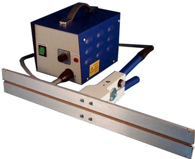
The sealing tong is heated on both sides so that also thick films can be sealed. Thermoplastic films of 2 x 0,025 up to 2 x 0,4 mm (PE) can be sealed with this equipment. The sealing pressure is achieved by a built-in spring, so that the pressure and the quality of the sealing is always equal. The sealing tong can be used for sealings at the edge of the film-material.
